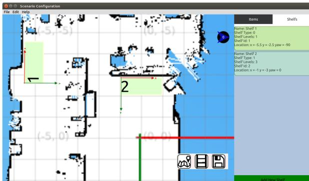
Fig. 3. Domain-specific software tool for modeling intralogistic environments. The GUI shows a map with two placed shelves.
