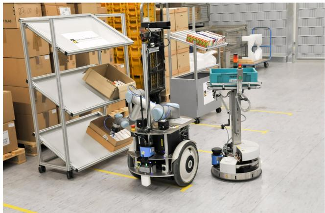
Fig. 1. Collaborative robotic commissioning, picking pharmaceutical packages from cardboard boxes in industrial environment.
