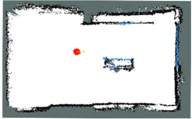
Fig. 1: An example of the localization with respect to a prior map based on AMCL using the ToF camera data is shown. Particles approximating the vehicle's pose (red), the estimated pose (yellow) and the 2D range scan (blue) projected from the ToF camera data are plotted. Note the large field of view of the camera which is not yet common for ToF cameras.
